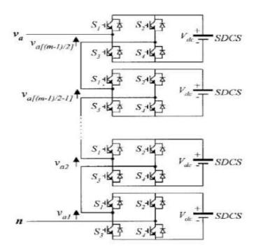
Fig.2 Single Phase 9 level H Bridge Inverter
