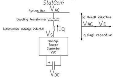
Fig.1 Schematic Configuration of STATCOM
